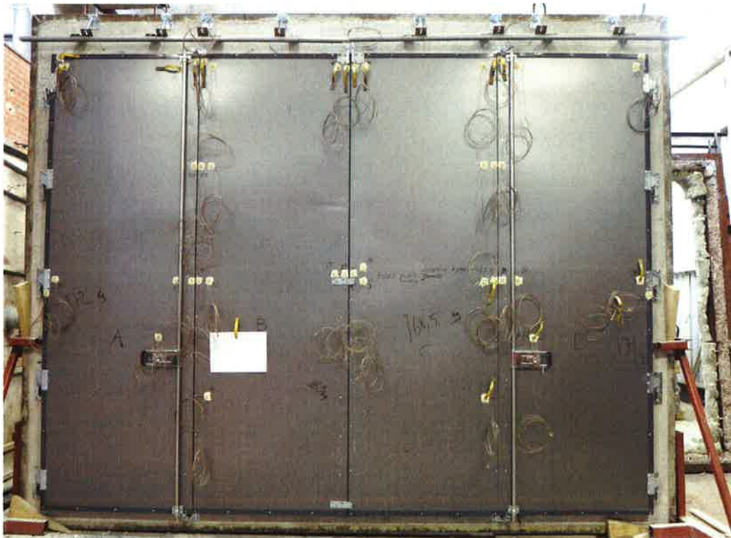
Figure 2. Unexposed side of the test specimen prior to the fire test.
