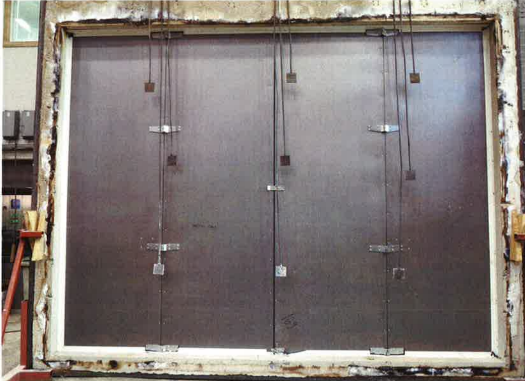
Figure 1. Exposed side of the test specimen prior to the fire test.
