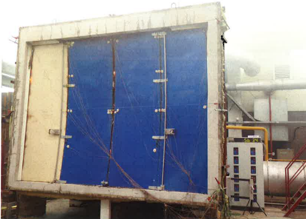
Figure 3. Unexposed side of the test specimen after the fire test.
