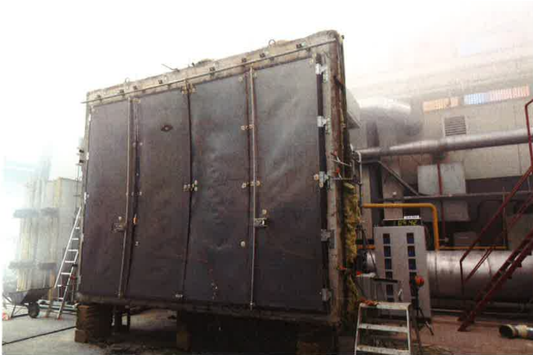
Figure 3. Unexposed side of the test specimen after the fire test.
