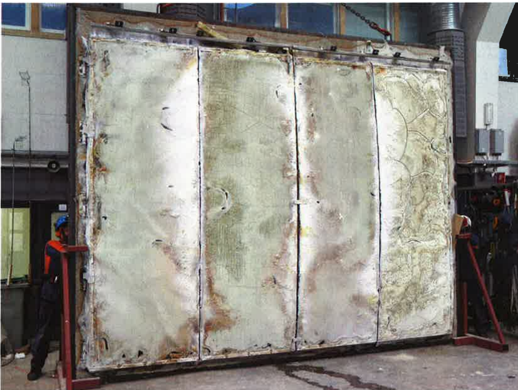
Figure 4. Exposed side of the test specimen after the fire test.
