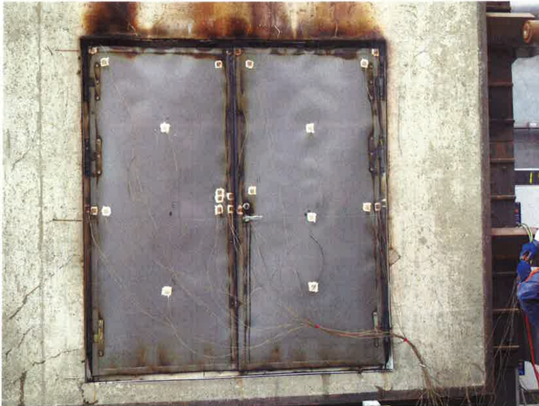
Figure 3. Unexposed side of the test specimen after the fire test.
